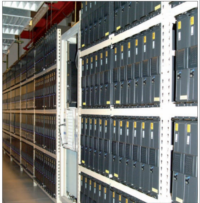
The Pion cluster at Fermilab consists of 520 Intel Pentium PCs.
