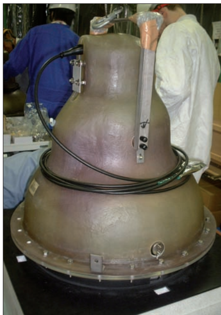
The 50 cm diameter PMTs are encased in a fibre-reinforced plastic cover to prevent a shock wave even if a PMT implodes again.
